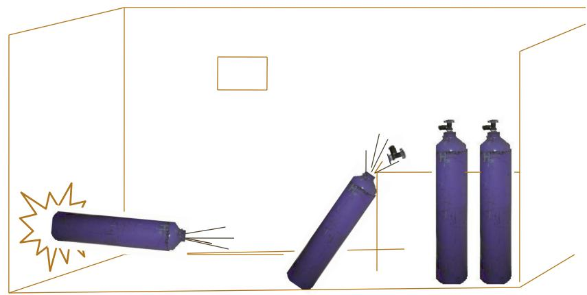
Gas cylinders should be capped when they are not connected to the system.
