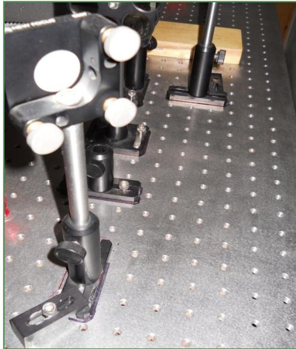
Secure optical components to the table to prevent stray reflections from misaligned optics.
